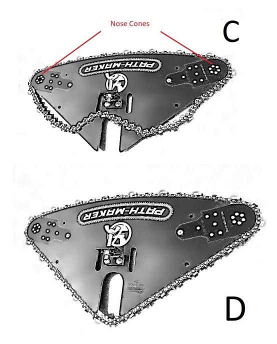
Once the chain is fully around the bar, and the guide teeth are properly in place (D), slip the chain around the clutch sprocket (E), ensuring that the guide teeth (F) are appropriately inside the sprocket.
